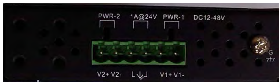
IES-2050A power connection
