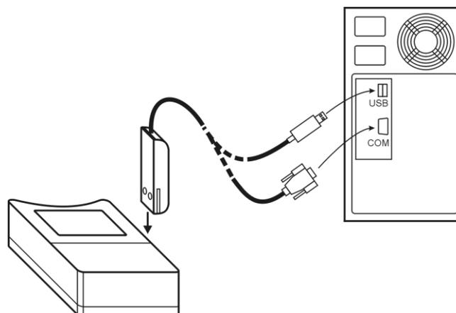
to use USB ADAPTER. Connect adapter connector to proper computer port and plug the adapter to the guide slots on the side of logger.
