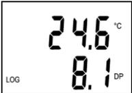
Every 5 s display is automatically switched to displaying of other measured or calculated quantity. Logger now displays ambient temperature and dew point temperature (LCD line marked by symbol DP).
