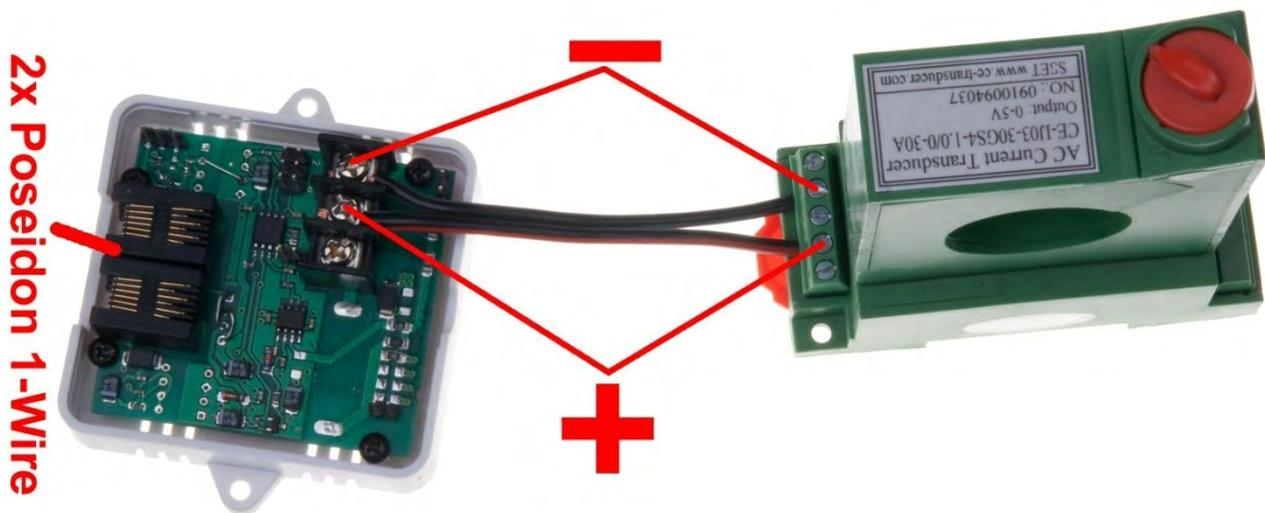
The polarity is indicated on both the probe and the converter. The NC terminal at the converter is not connected.
